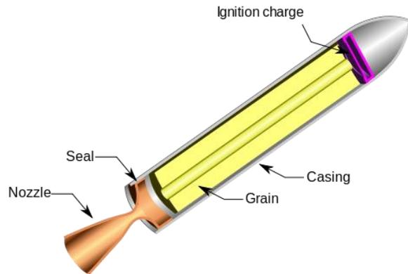
**Solid Rocket Motor System Diagram**
