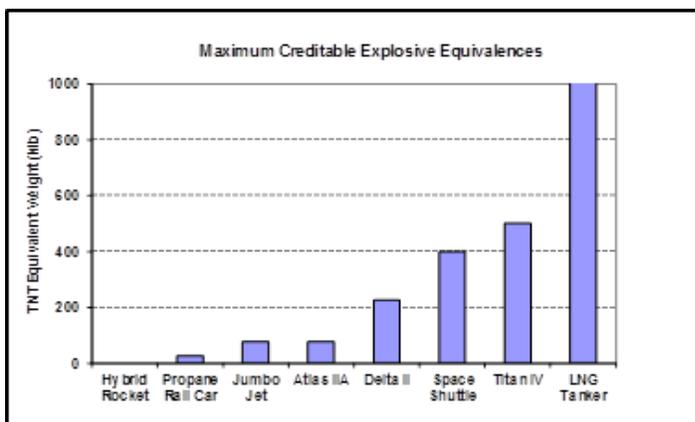
bullet. Highly energetic chemicals like those used in rockets can be very volatile and explosive. To dramatize this point, the graph (left) compares the explosive potential (TNT equivalence) of several orbital launchers with other transportation vehicles carrying highly energetic fuels. Note also the “0” TNT equivalency for Hybrid Rockets (to the left on the graph) which will be discussed later.
