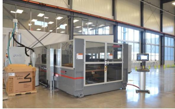
D-DART Fuel Grains Being 3D Printed on the Big Area Additive Manufacturing (BAAM) Machine – Courtesy Cincinnati, Inc.
